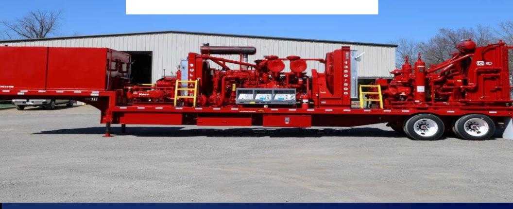
Foam Air Unit (FAU) field unit comprised of water pump, surfactant/chemical pump, and air compressor
