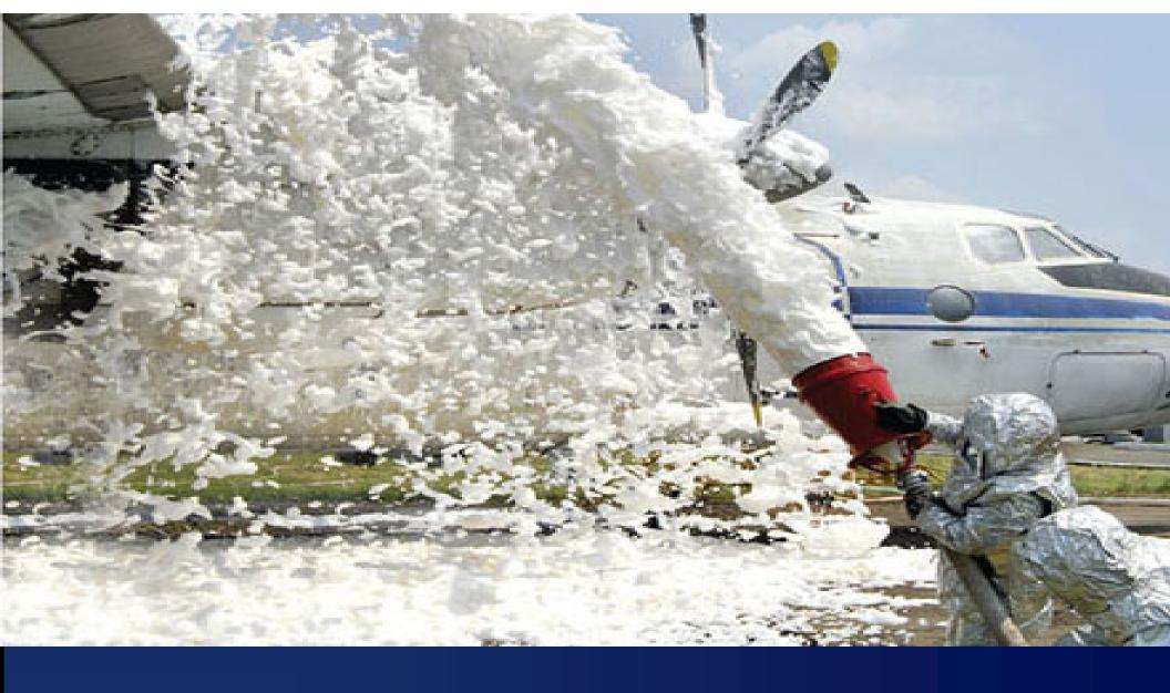
Foam air is used to extinguish fires, especially aviation fuel.
