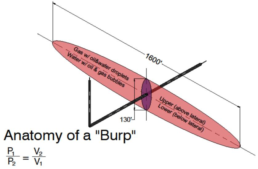
If bottom hole circulating pressure drops by 10 PSI, from 1,900 PSIA to 1,890 PSIA
