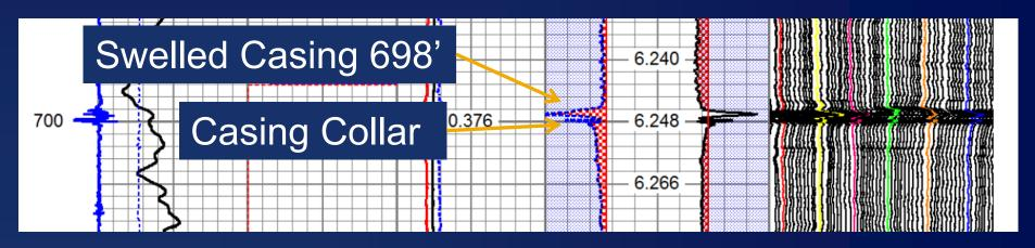
Casing swelled at depths of tubing deformations. Casing passed a pressure test after the incident.
