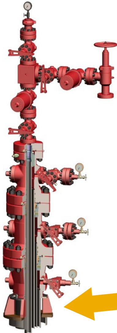
To the Production wing valve or associated flange
