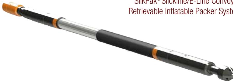
SlikPak is a battery-powered assembly that can run 2.13 in. to 14.5 in. inflatable bridge plugs or packers. The inflation fluid can be obtained from the wellbore or carried in adaptable fluid chambers. SlikPak is ideal for remote locations or wellsites with a small footprint.
